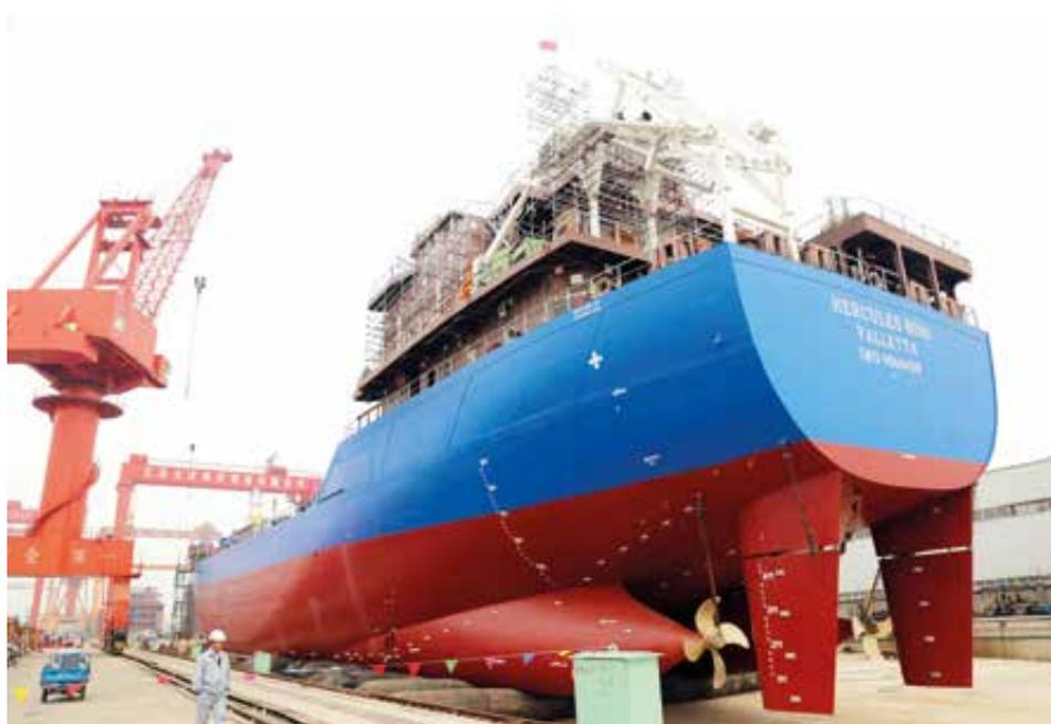
**'Hercules 8000' is fitted with twin propellers and rudders for extra manoeuvrability**
